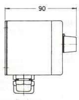
Sensor dia. 6 mm Capillary tube dia. 1,5 mm 1,0 m long Weight 1,4 kg
