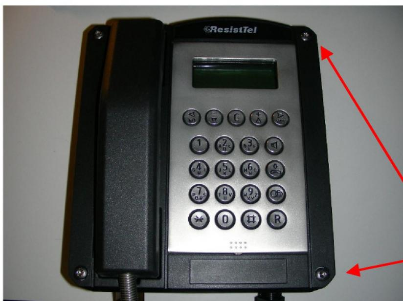
Put upper part of telephone onto the lower part of the telephone and fasten with 4 cover screws (torque 3Nm, key TX30)
