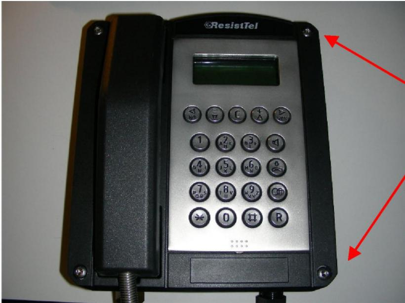
Loosen 4 cover screws with torx key TX30.
