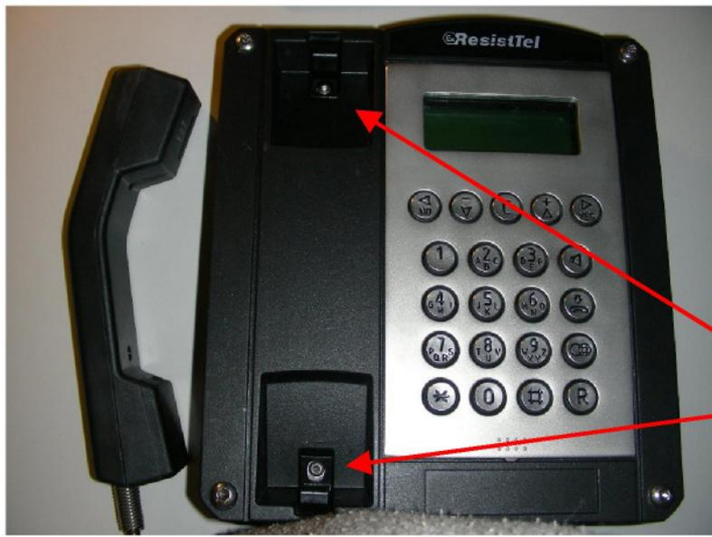
Remove handset from the upper part of the telephone. Loosen screws for fastening the receiver hook using a key Tx20. Remove receiver hooks on both sides of the telephone upper part.
