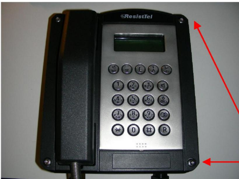
Put upper part of telephone onto lower part of telephone and fasten with 4 cover screws (torque 3Nm, key TX30)
